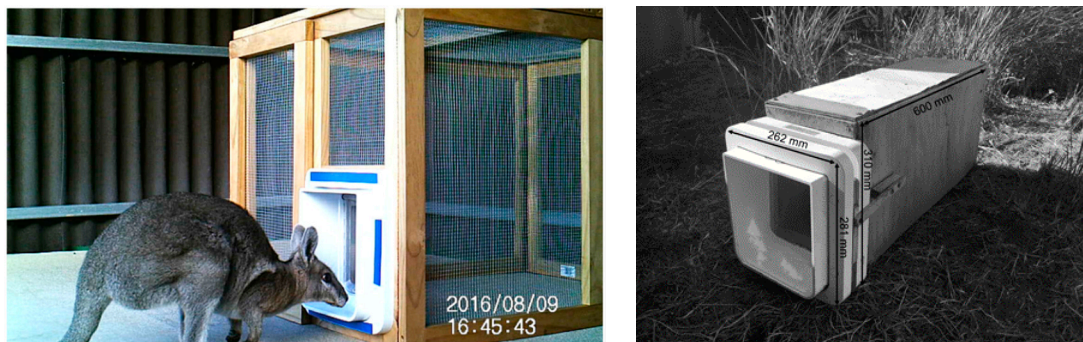
Figure 10. (Left) commercially available Sure Petcare RFID microchip controlled pet door adapted for use as a wildlife provisioning station and refuge with a bridled naitail wallaby (Photo: S. Muns) [56]. (Right) Prototype microchip controlled nest box used with northern brown bandicoots (Photo: M. Edwards) [39, 59].
